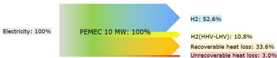
Figure 27 - The energy inputs from and outputs of a PEMEC (2020, 10MW hydrogen plants). Data is derived from Ramboll references.
