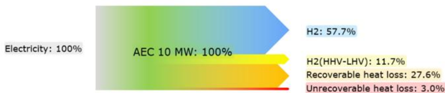
Figure 26 - The energy inputs from and outputs of an AEC (2020, 10MW hydrogen plants). Data is derived from Ramboll references.
